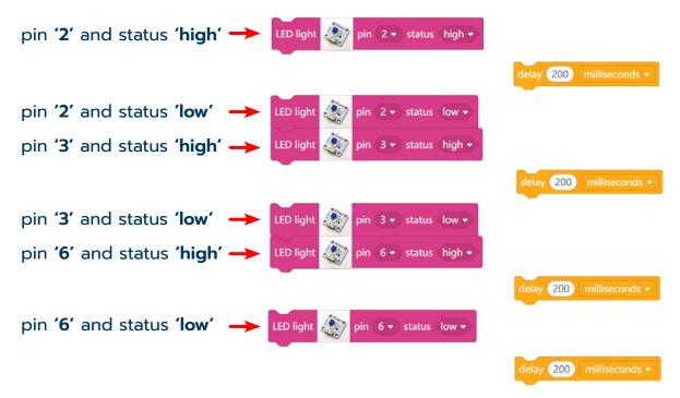
Then, set the four 'delay ()' blocks to 200 milliseconds.
