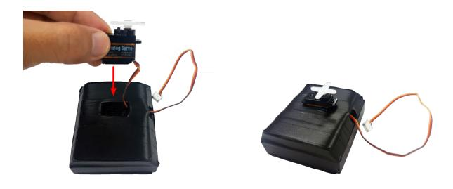
Secondly, install the servomotor upper bracket on the top of the first servomotor (via servomotor arm), then secure it with the screw.
