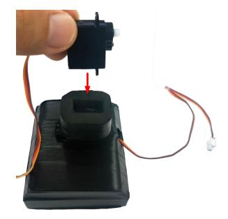
Fourth, install the VIA Pixetto onto the camera bracket then install the camera bracket onto the first servomotor, and secure it with the screw.
