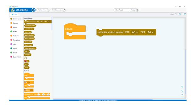
Place it within the 'setup' block. This block will relate information to the VIA Pixetto vision sensor.
