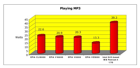
Power consumption of the VIA EPIA CL10000 is around 70% that of the reference platform
