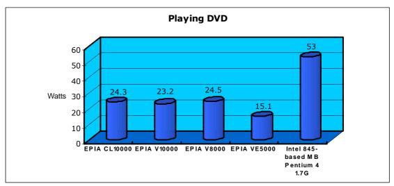
The power consumption of the VIA EPIA CL10000 is more than half of that of the reference platform.
