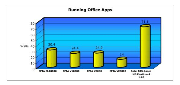
The comparison above uses CC Winstone 2001 to compare power consumption while carrying out standard office tasks like word processing, manipulating spreadsheets and web browsing. In this comparison, the VIA EPIA CL10000 mainboard uses more than 50% less power than the reference platform.
