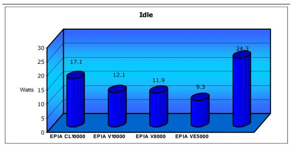
In this comparison, the power consumed while standing idle is compared and the VIA EPIA CL-Series mainboards draw around 70% of the power that the reference platform draws.
