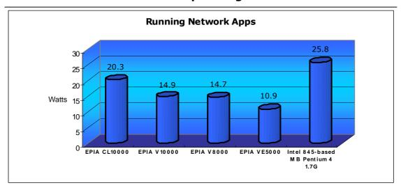
The power consumption comparison for network applications was run while transferring large data files over a standard 10 Base T network. Here again the power consumption of the Intel reference platform is considerably more than that of the VIA EPIA series of Mini-ITX mainboards.
