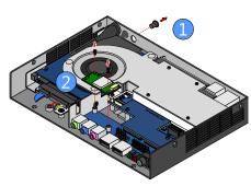
Step 2 Remove the P910-D bridge board connector.
