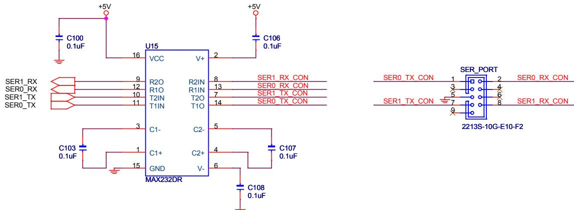
Figure 42: Serial COM port Interface Example
