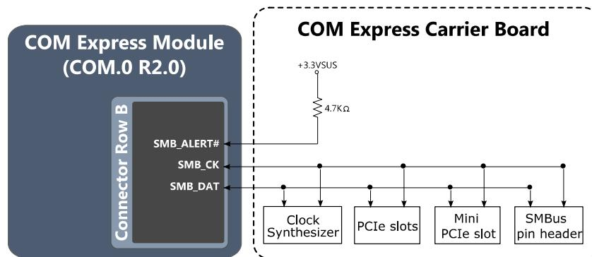
Figure 63: SMBus Interface Example
