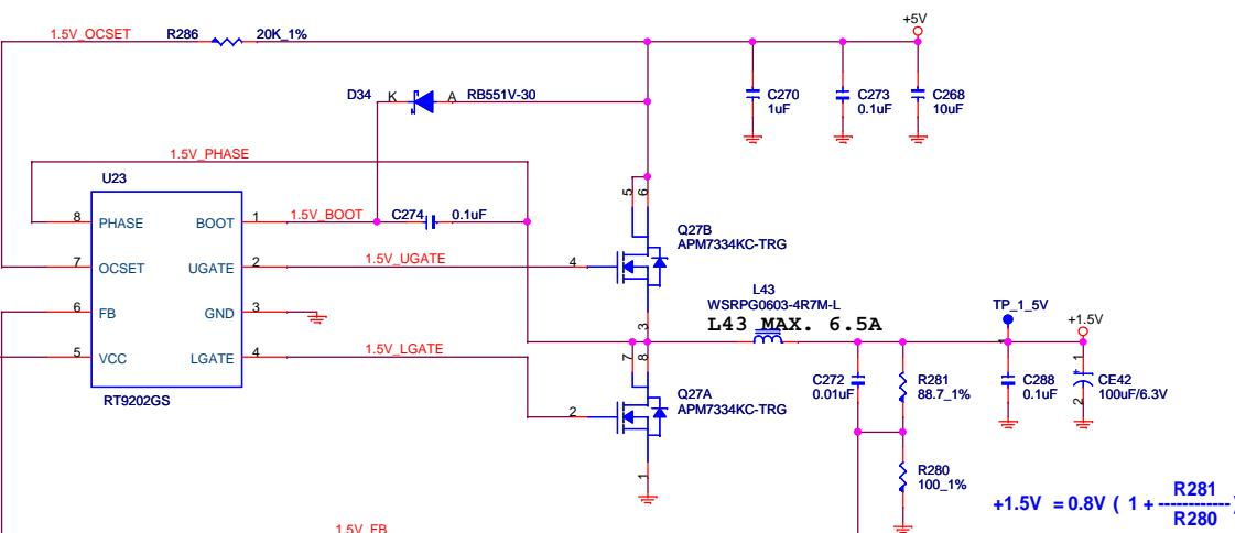
For Mini-PCIe Slot +1.5V
