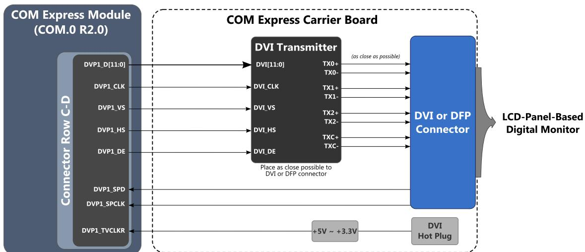
Figure 36: Digital Panel Interface using External DVI Transmitter Implementation
