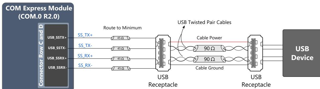
Figure 57: USB 3.0 Differential Signal Layout Recommendations
