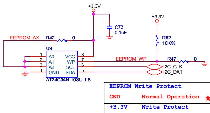
Figure 44: EEPROM Circuitry Reference Example
