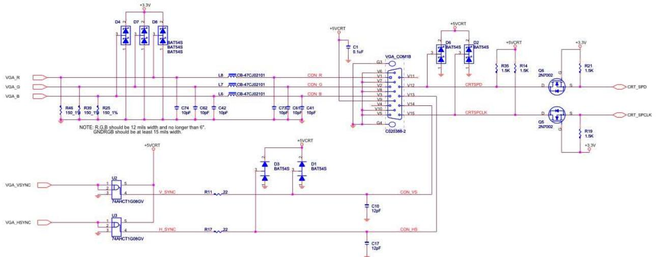
Figure 26: VGA Interface Connector Example
