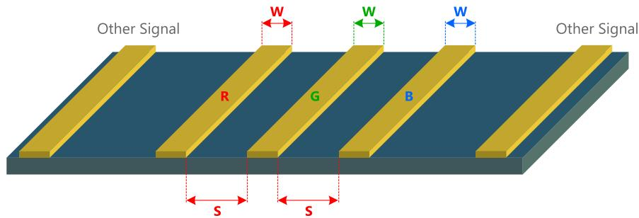
Figure 28: Recommended RGB Trace Properties
