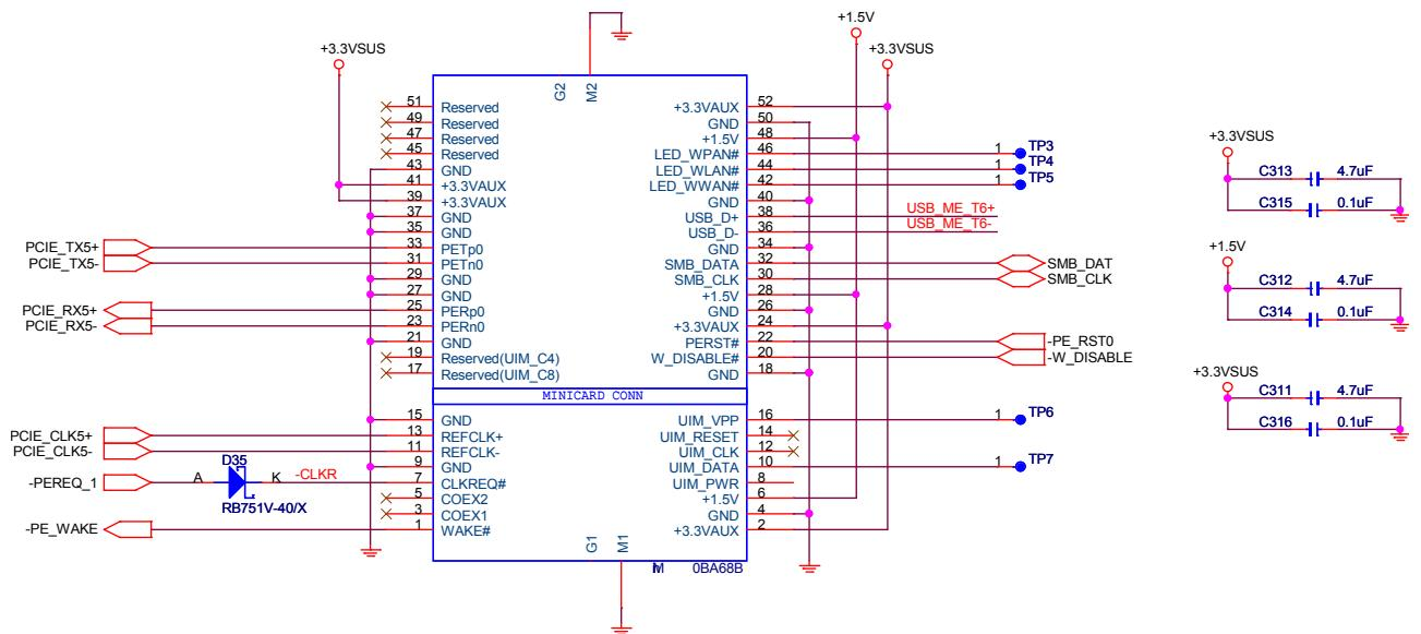
Figure 17: Mini PCI Express Card Socket
