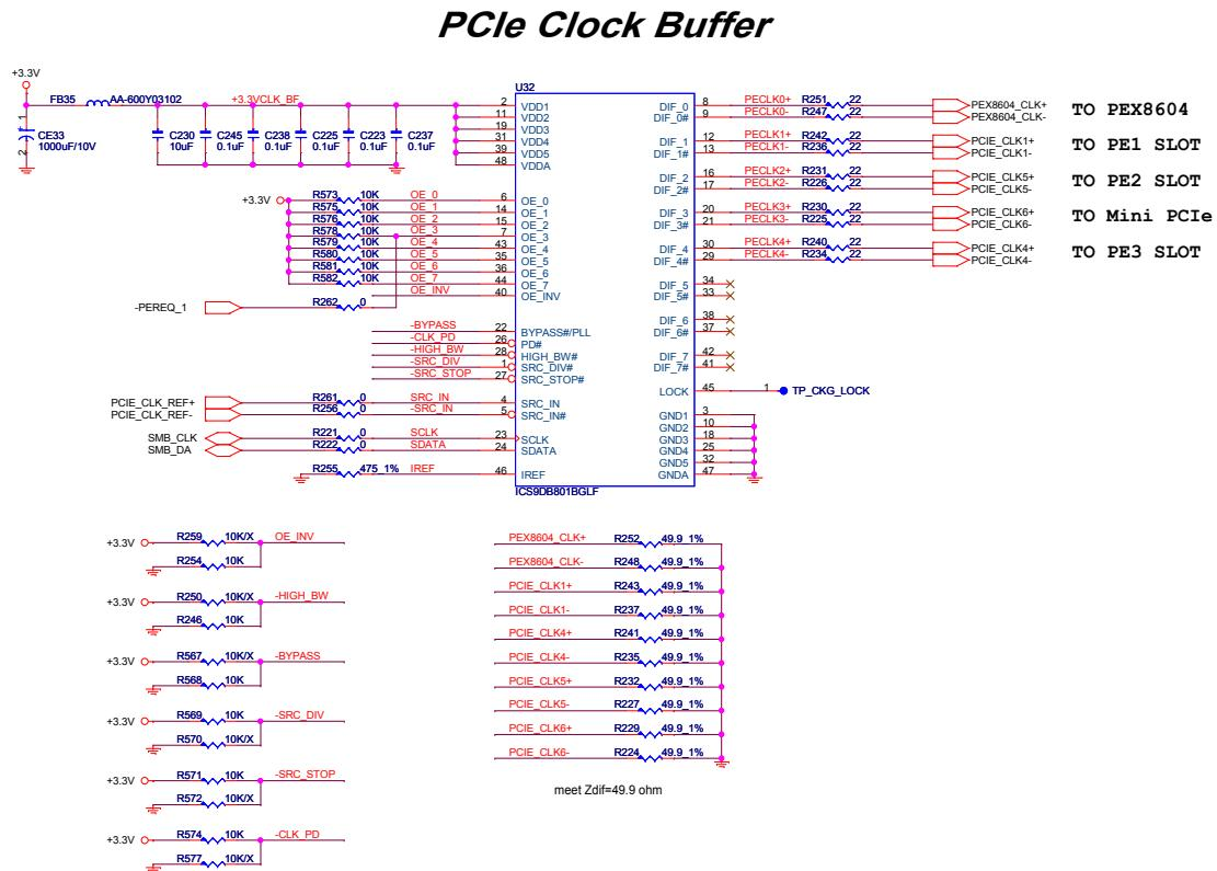
Figure 14: PCI Express Clock Buffer
