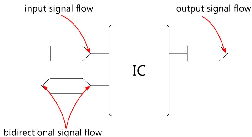
Figure 1: Conventions pertaining to illustration and schematics
