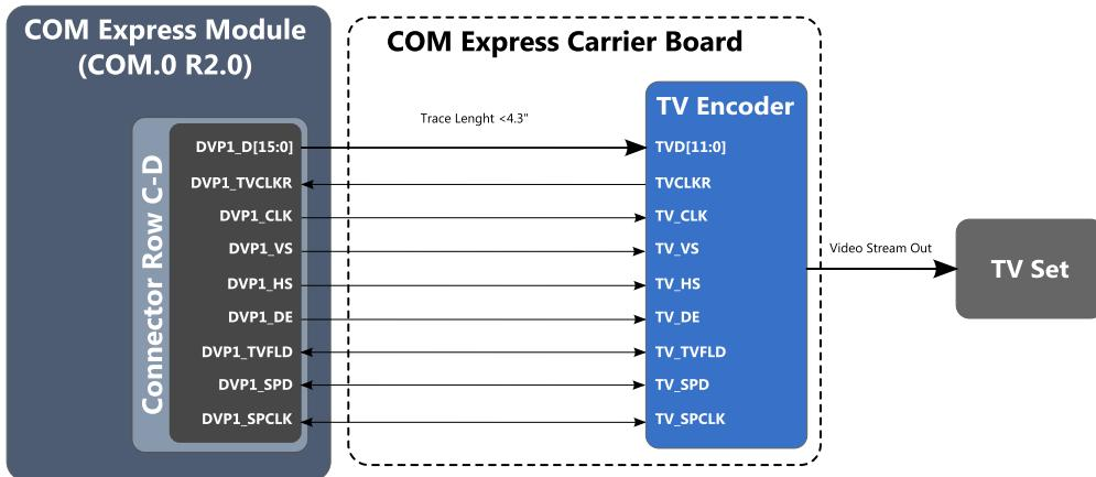
Figure 35: Digital TV-out Interface using External TV Encoder Implementation
