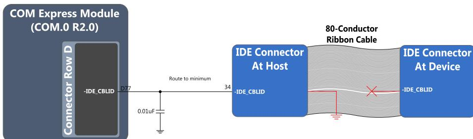
Figure 51: IDE Cable Detection with 80-Conductor Ribbon Cable
