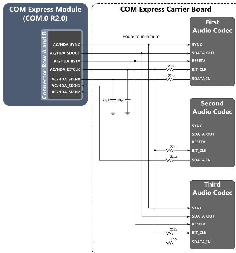
Figure 62: Fully On-Board High Definition Audio Codec Implementation Example
