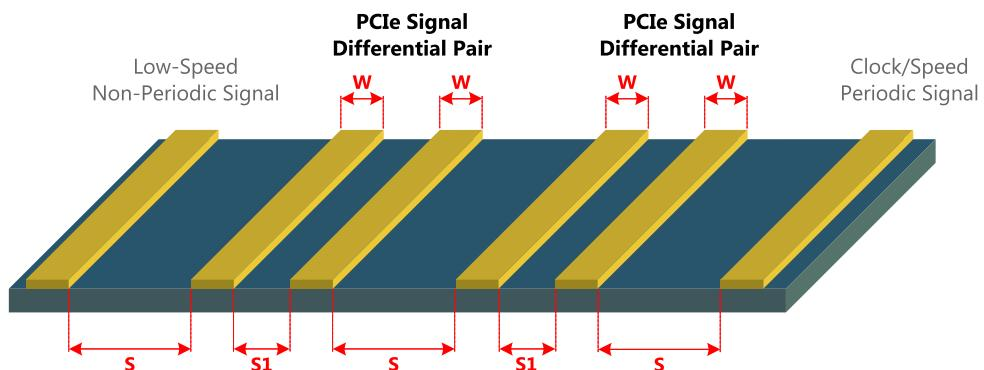
Figure 22: PEG x4 Trace Spacing
