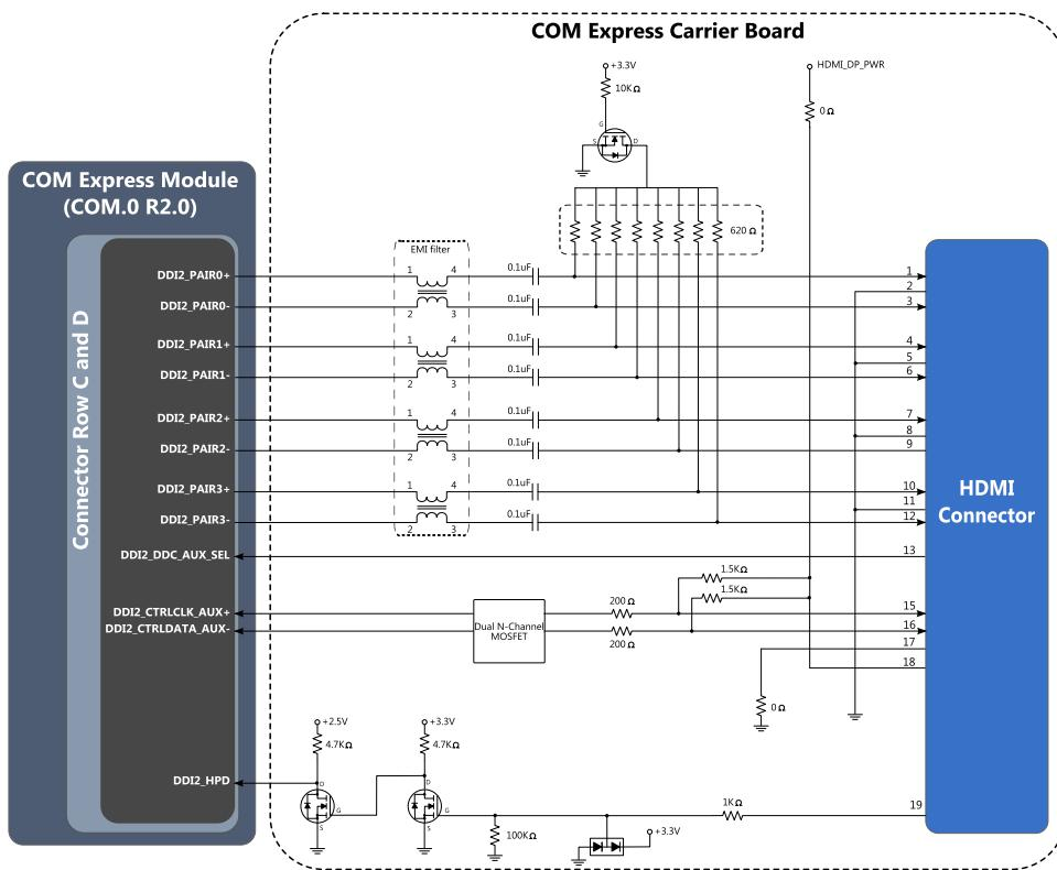
Figure 24: HDMI® Interface Connector Diagram
