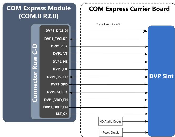
Figure 34: DVP Slot Interface Diagram
