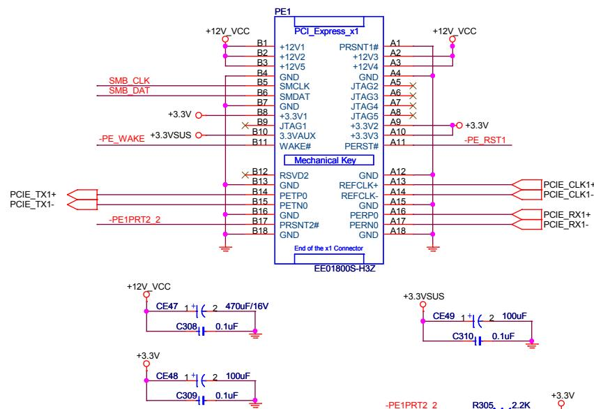
Figure 15: PCI Express x1 Mode Slot
