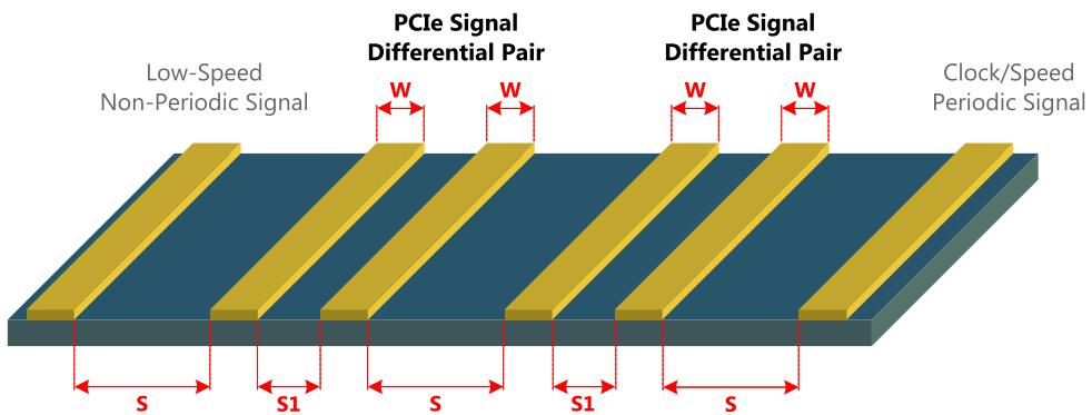
Figure 19: PCI Express (x1 mode) Trace Spacing
