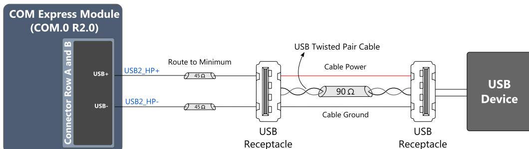
Figure 56: USB 2.0 Differential Signal Layout Recommendations
