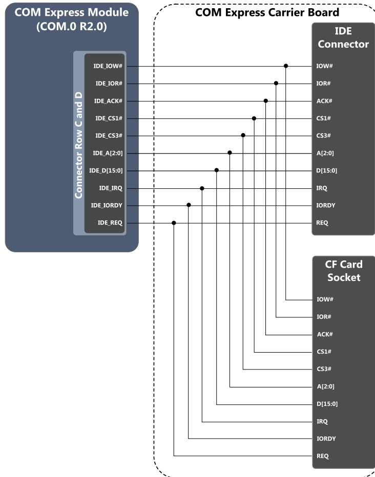
Figure 49: IDE Devices Layout Guidelines
