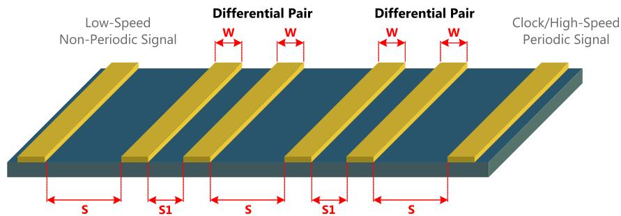
Figure 59: USB 2.0 and 3.0 Trace Spacing
