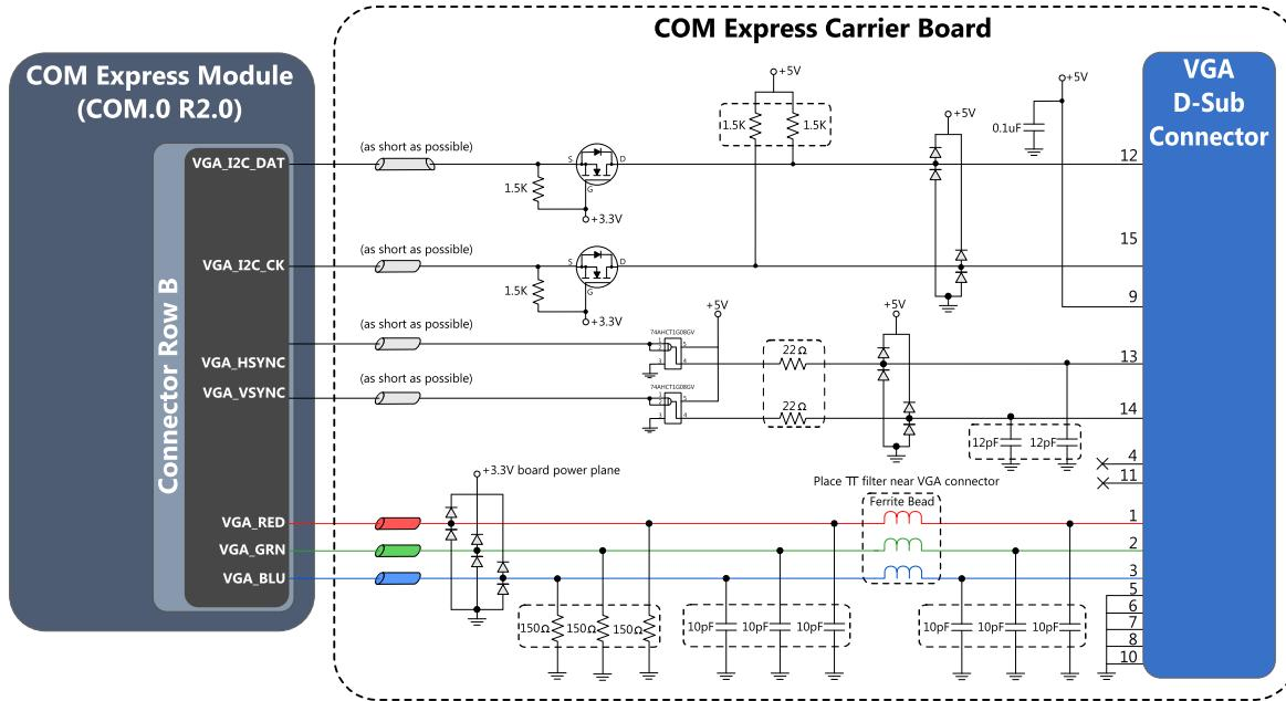
Figure 27: VGA Interface Sample Diagram
