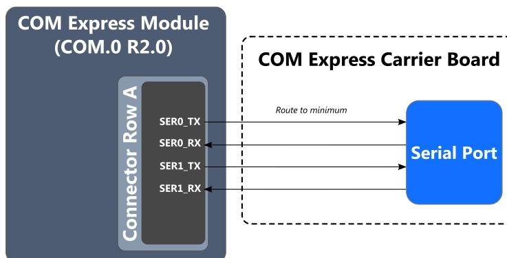
Figure 43: Serial COM port Interface Topology Example
