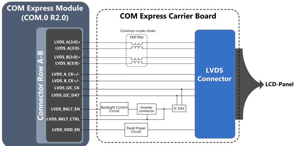
Figure 32: LVDS Interface Sample Diagram
