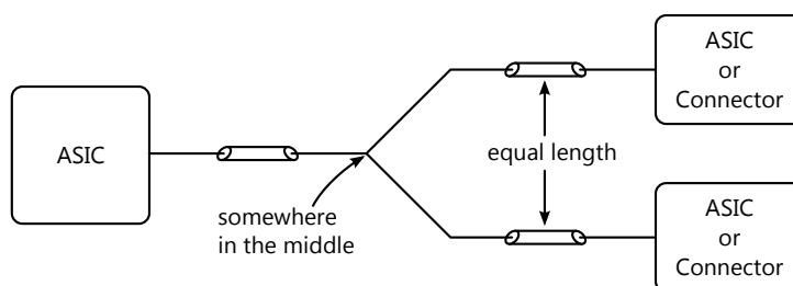
Figure 6: Alternate multi-drop example
