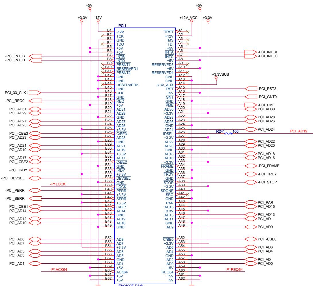
Figure 45: PCI Connector Example
