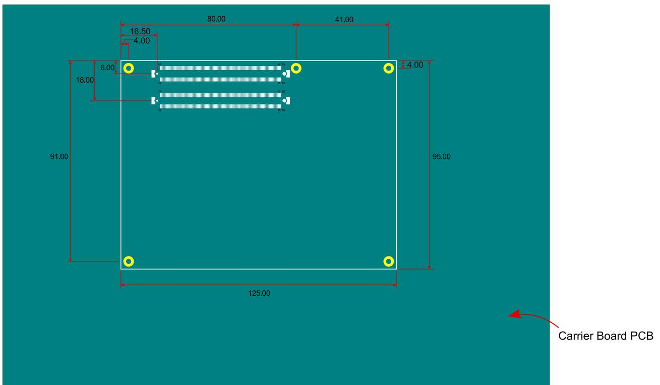
Figure 10: COM Express connector placement on Carrier Board PCB
