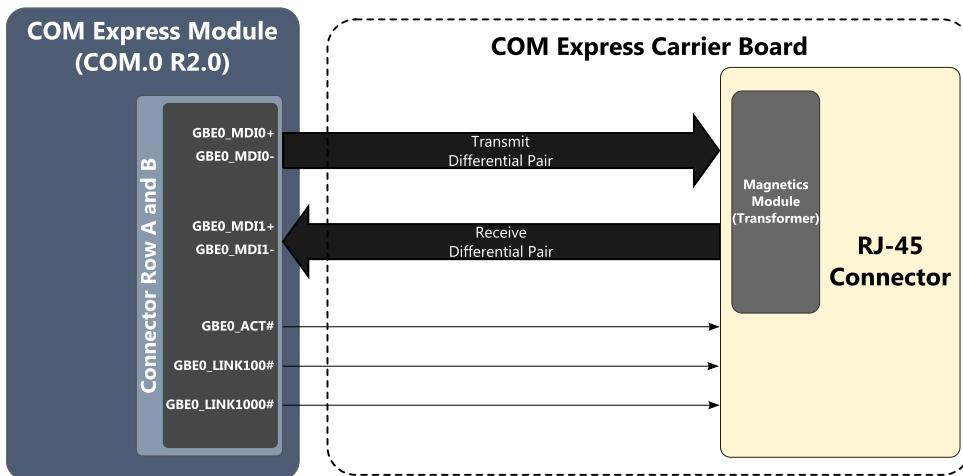
Figure 65: 10/100 Ethernet Layout Recommendation (integrated magnetic module)
