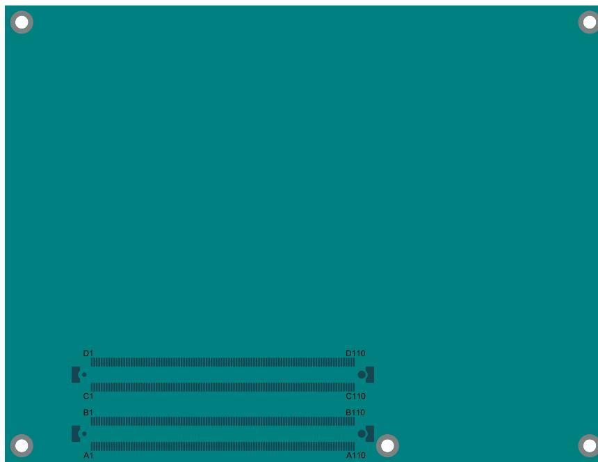
Figure 13: Orientation of COM Express connectors on a COM Express module
