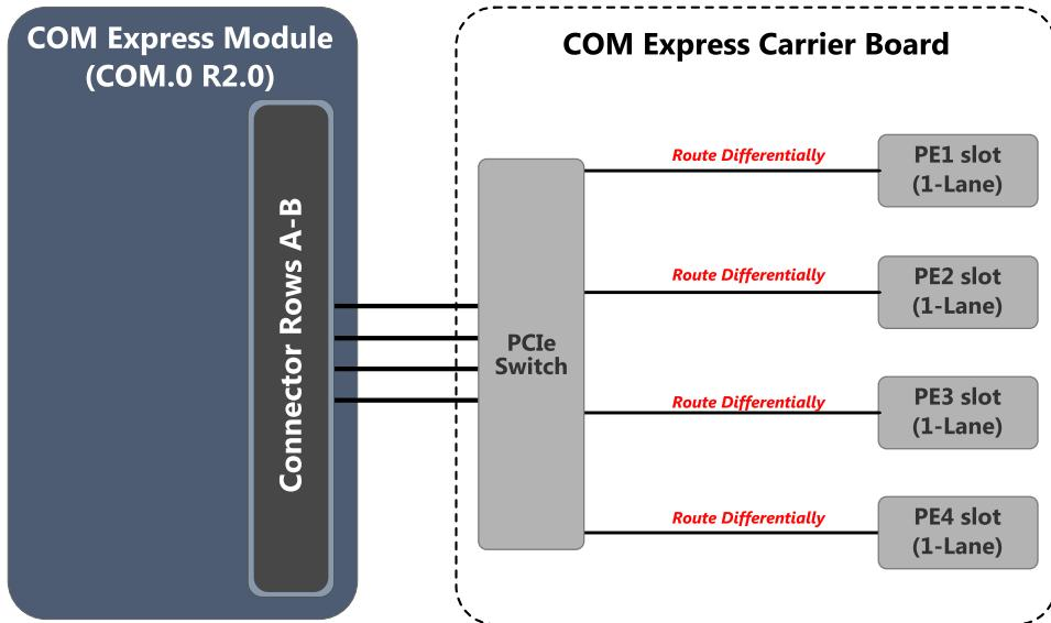
Figure 16: PCI Express x1 Mode Topology Example
