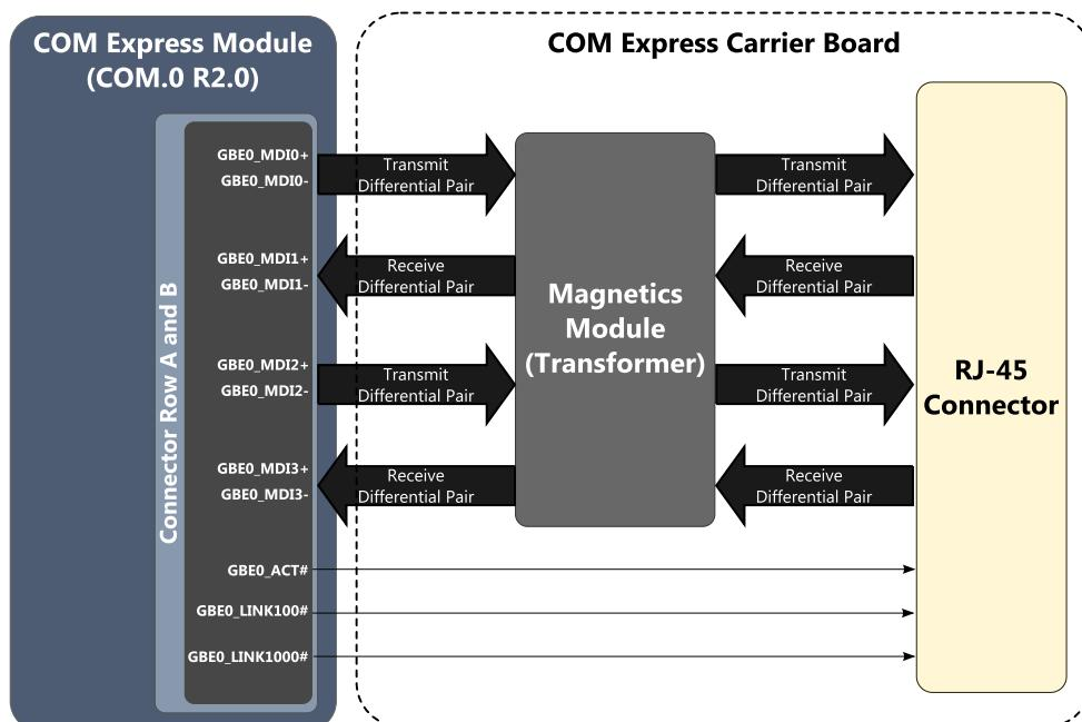
Figure 68: Gigabit Ethernet Layout Recommendations (external magnetic module)
