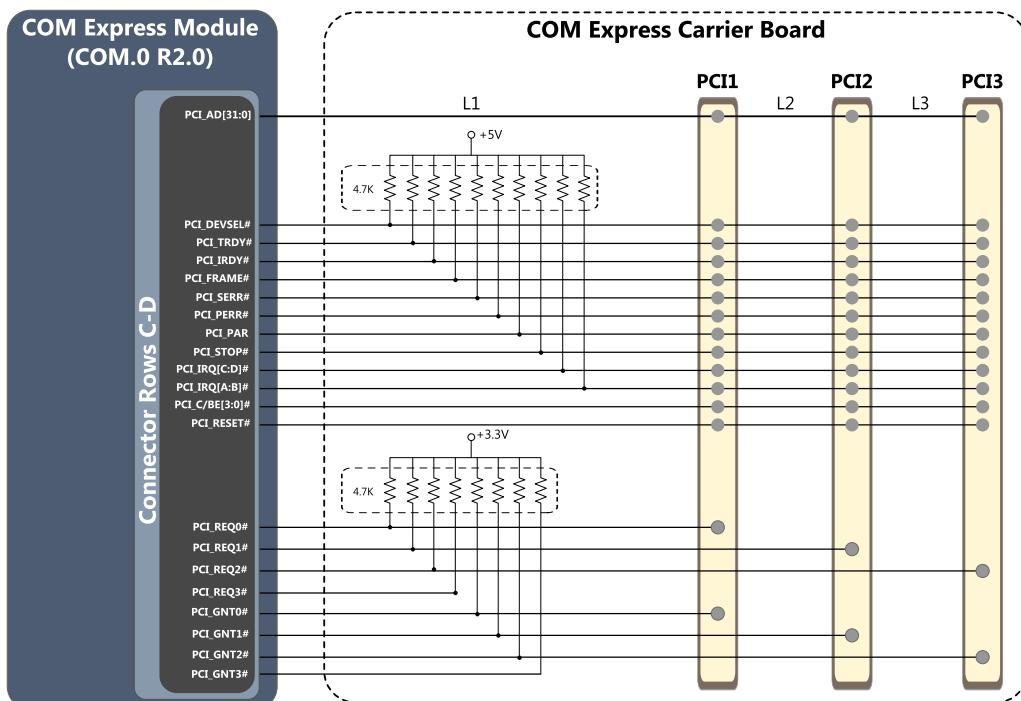
Figure 46: PCI Interface Topology Example
