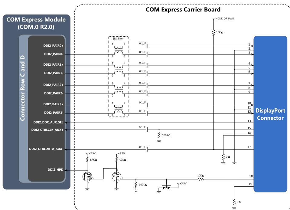
Figure 25: DisplayPort Interface Connector Diagram
