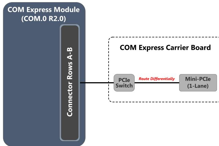
Figure 18: Mini PCI Express x1 Mode Topology Example
