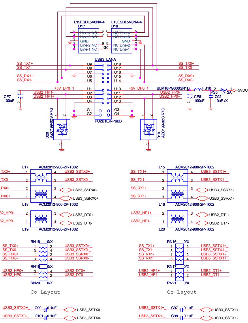
Figure 55: USB 3.0 (port 0 and port 1) Interface
