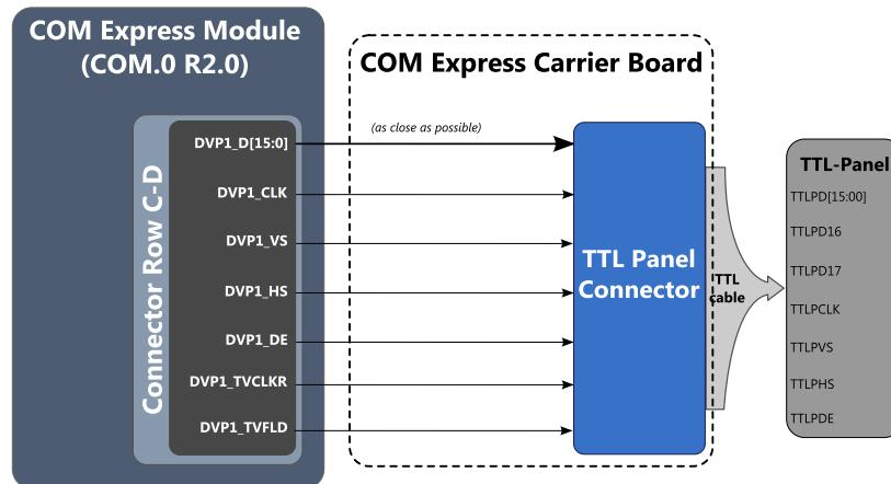
Figure 37: TTL Panel Interface using External TTL Panel Implementation
