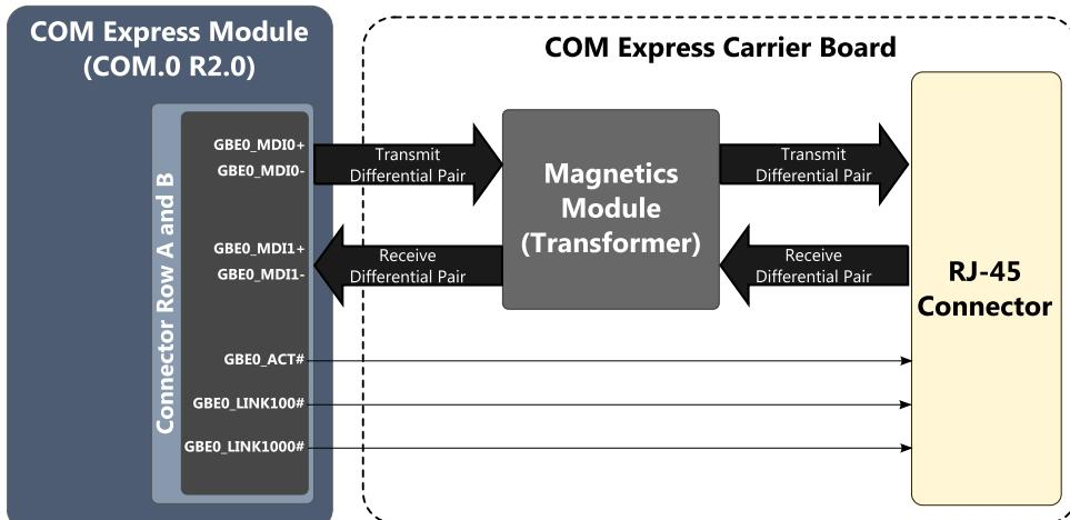
Figure 66: 10/100 Ethernet Layout Recommendation (external magnetic module)
