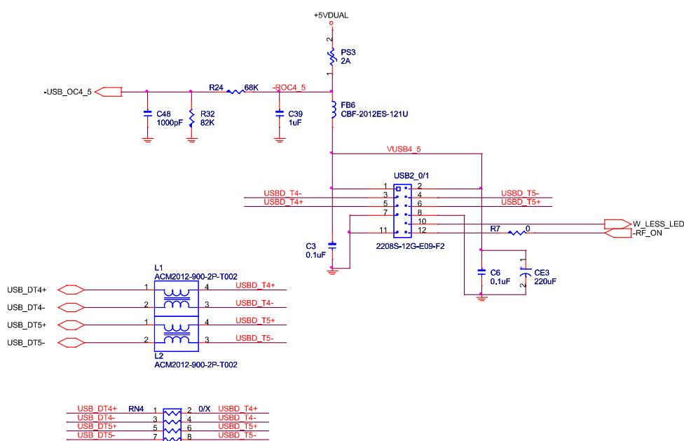
Figure 54: USB 2.0 (port 0 and port 1) Interface
