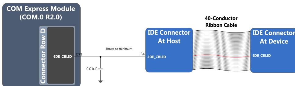
Figure 50: IDE Cable Detection with 40-Conductor Ribbon Cable
