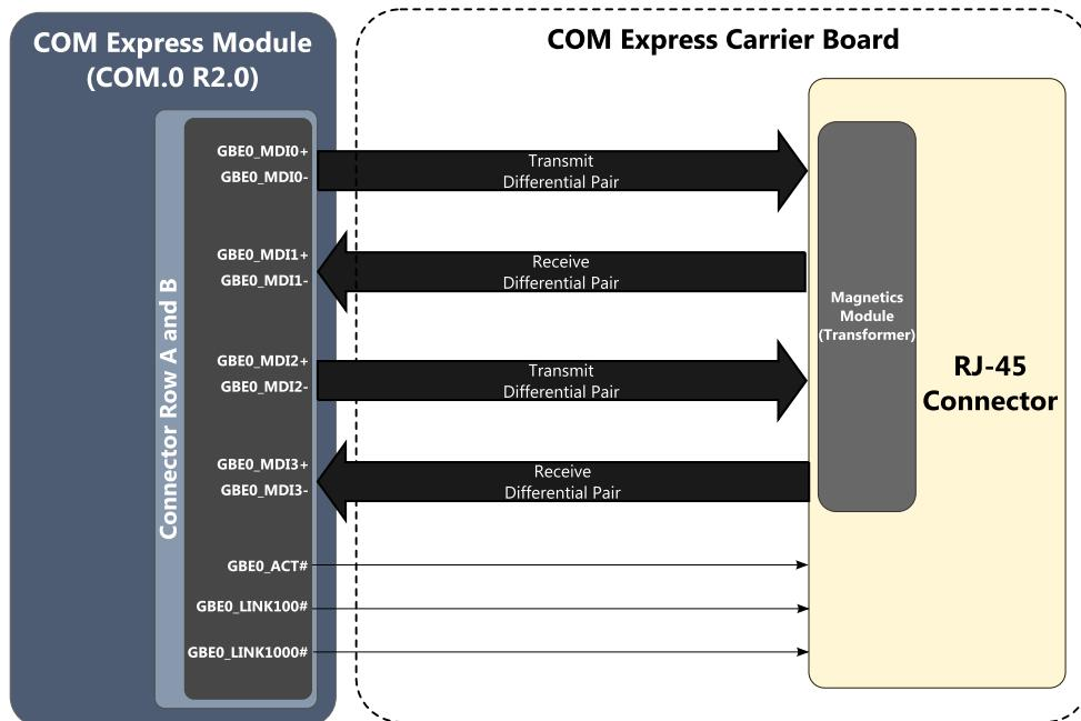
Figure 67: Gigabit Ethernet Layout Recommendations (integrated magnetic module)
