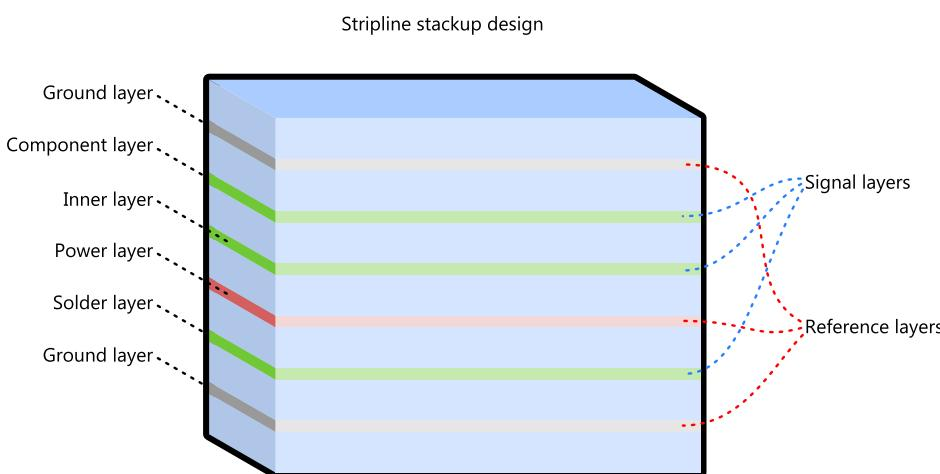
Figure 3: Six-layer stripline PCB stackup example
