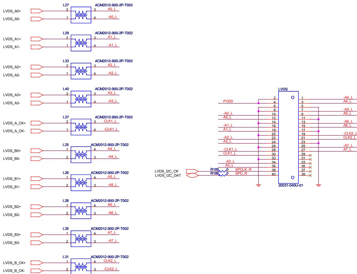
Figure 29: LVDS Connector Example
