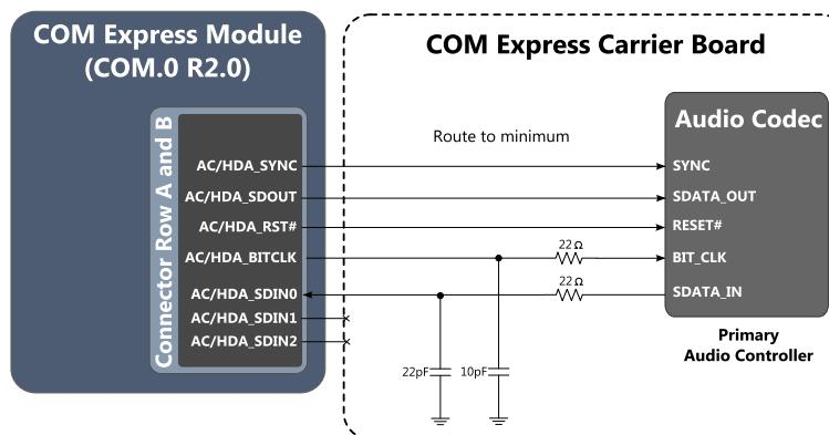
Figure 61: Single On-Board High Definition Audio Codec Implementation Example
