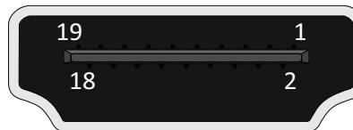
Figure 38: HDMI port diagram
