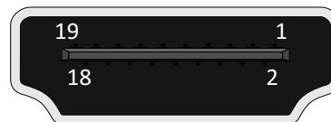
Figure 34: HDMI port diagram
