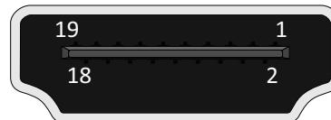
Figure 34: HDMI port diagram
