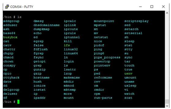
"dmesg" is the command to display all messages from the Linux kernel ring buffer.
