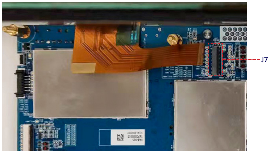
Figure 47: Connecting the 39-pin FFC cable of the TFT-LCD display to 'J7'
