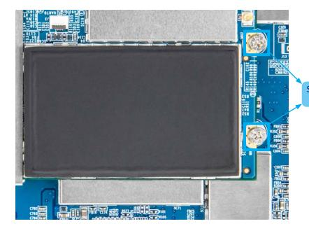
Screws inserted to secure SOM-9X35 Module on Carrier Board
